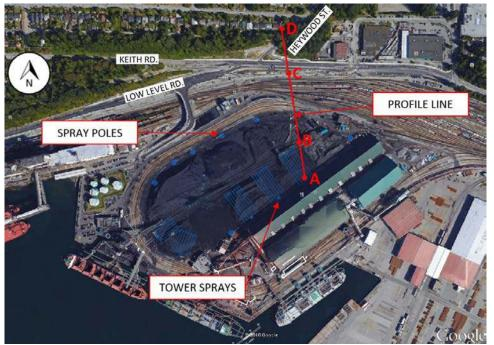
The drop distance from the Tower Spray nozzles will be approximately 40 m above ground at its base.
