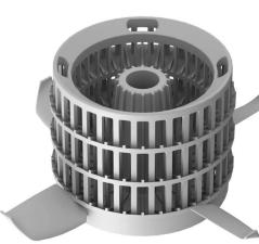
EK's droplet spectra have the highest industry average between 20-80 microns. Creating this much surface area allows for a faster evaporation rate and lowers the typical pond size requirements by a 10 to 1 ratio. Rotary atomization enables the manipulation of droplet sizes by changing the speed of the atomizer that allows control during any overspray conditions.
