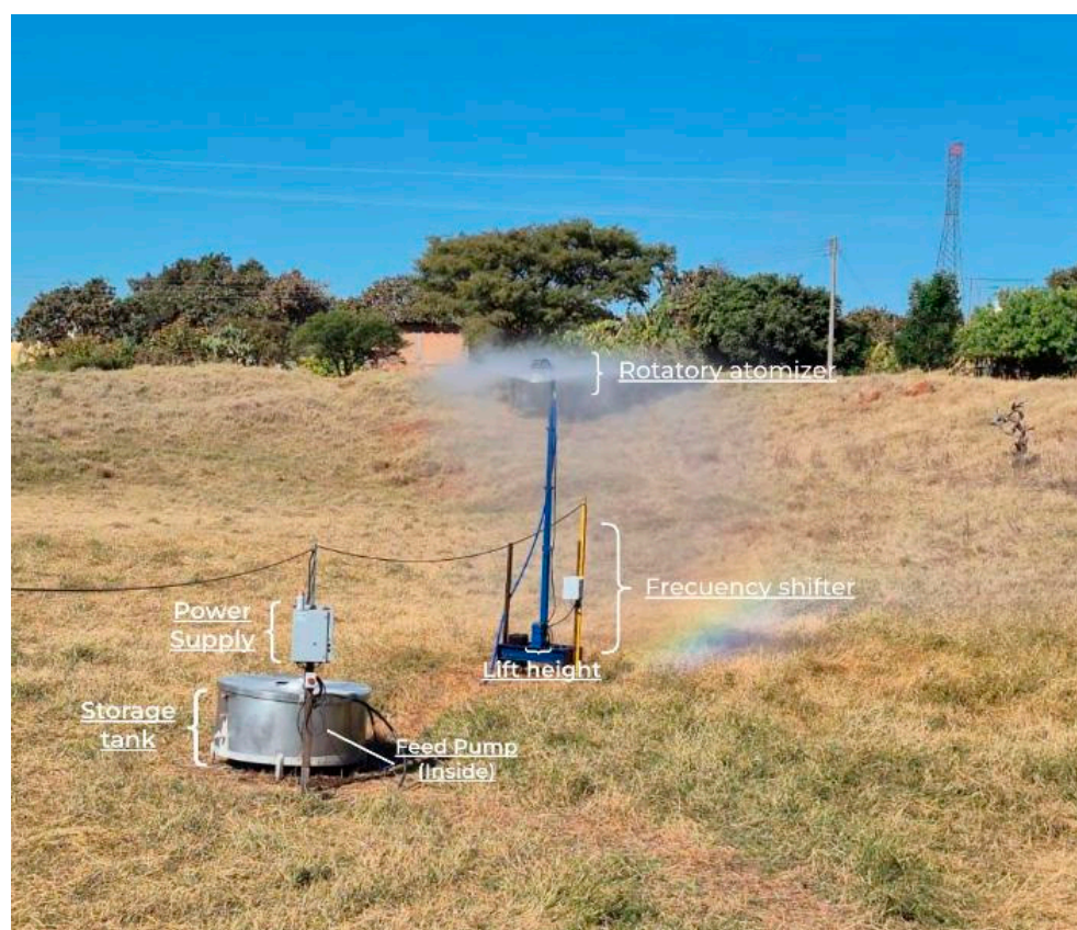
Figure 2. Photograph of the experimental droplet evaporation equipment.
